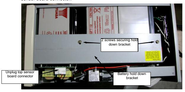
8. Remove the third screw securing the battery hold-down bracket (see detail picture)
