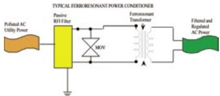
1. Passive RFI Filter minor line noise and RFI.
