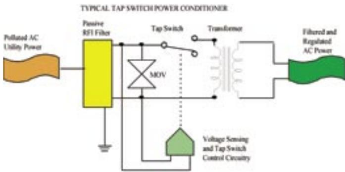
1. Passive RFI Filter minor line noise and RFI.
