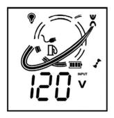
When green mode is activated, the UPS will automatically transfer to bypass mode once the connected load drops to less than 3% of the UPS's rated output. The load will operate directly from utility power. The LCD will indicate the UPS is in bypass mode and the green mode bulb icon will be flashing. If the load is increased to over 3% of the UPS output rating, the system will automatically transfer back to normal, on-line operation.
