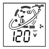
Online mode operation indicates the load, inverter, PFC, line, charger and battery status. The fan is shown at medium speed.
