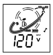
Bypass mode indicates the input is connected directly to the load. The dark solid line shows the input power to the battery charger icon, then to the battery. The fan is shown in low speed mode.
