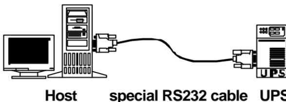
1. Connect the DB-9 male connector of the cable to the UPS interface. (A DB-9 female connector of RS232 protocol type.).
